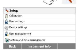
Press the **Setup** button to access Setup menu.
