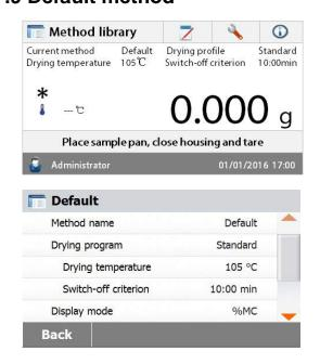
The analyzer comes with a default method preinstalled.
