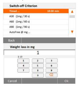
Select AutoFree mean weight loss per unit of time or weight loss in percent per unit of time.
