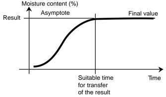
In the second type, drying runs quickly at the start and then flattens out. The moisture content never assumes a constant value. The causes of such a drying profile can be as follows:
