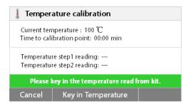
This is a two-point adjustment (100°C and 160°C). The dryer unit now heats to the second temperature (160°C). Adjustment of the temperature is defined by two points. Proceed exactly as you did for the first temperature. After you have set the display to agree with the thermometer, then press the **Enter** button.
