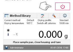
To **switch the Moisture Analyzer on**, press the **On/Off** button. An internal diagnostic test is performed; the display lights and the Home screen appears followed by the initial display.
