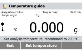
Press the **Set Temperature** button to enter the temperature setting.
