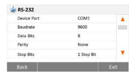
Select the following items to set RS232 port when RS232 port link to printer or other RS232 compatible device.
