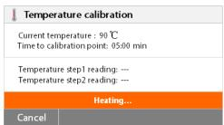
The dryer unit is heated to a temperature of 100°C. You can observe the progress on the display as the dryer temperature and count down period are displayed. After 15 minutes, read the thermometer through the inspection window on the cover and enter this temperature. Adjust the display reading to agree with the thermometer, then press the Enter button. You have 15 minutes to make this adjustment, otherwise the calibration is terminated.
