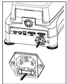
Using a test pen, turn the fuse holder to the left (counterclockwise) and remove the fuse.
