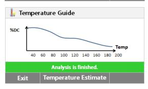
The analysis will finish with a characteristic curve calibrated by a temperature axis. Press **Temperature Estimate** button to compare the result curve with typical curve guide.
