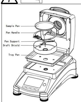
Open the cover and remove the pan handler, sample pan, draft shield, and heat shield from the instrument before cleaning.
