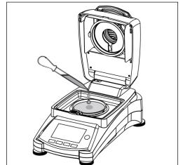
Wet the glass fiber pan with a 0.5 to 1 gram of water. Attention: Minimum sample size must be greater than 0.5 gram.
