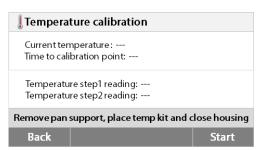
You are now prompted to remove the pan support. Place a temperature calibration unit and close the upper housing.
